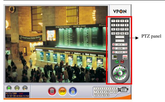
**PTZ panel:** You can do preset and recall, zoom in/out, focus, iris control to current camera. **Preset buttons-** Save current camera position. You can save totally16 preset positions
