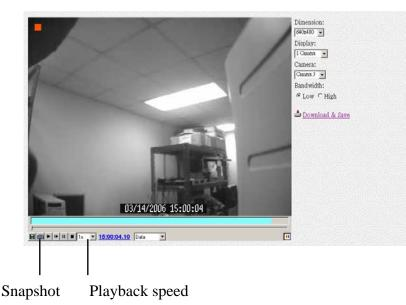
**Note:** The **playback start** time can be changed to jump to any time during the recording. Click on the **playback start** time and change the time using the keyboard.
