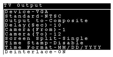
Use the **Up** and **Down** arrow buttons on the remote control to select any one of the displayed parameters and use the **Left** and **Right** buttons to cycle through the available options. Press the **OK** button when parameters are set correctly.
