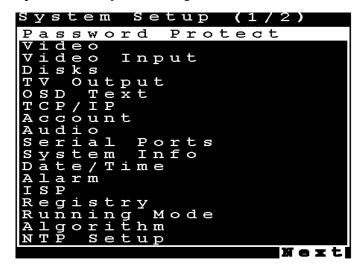
Use the Up and Down arrow buttons to highlight an option, and use the OK button to confirm your
