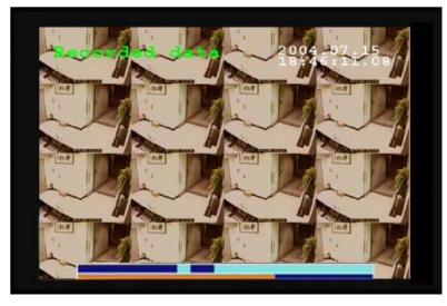
**GPI** - The screen shows where alarm triggers were generated. The red bar shows the trigger. To move to the next motion detection or alarm trigger event, press the **Right/Left** arrow buttons.
