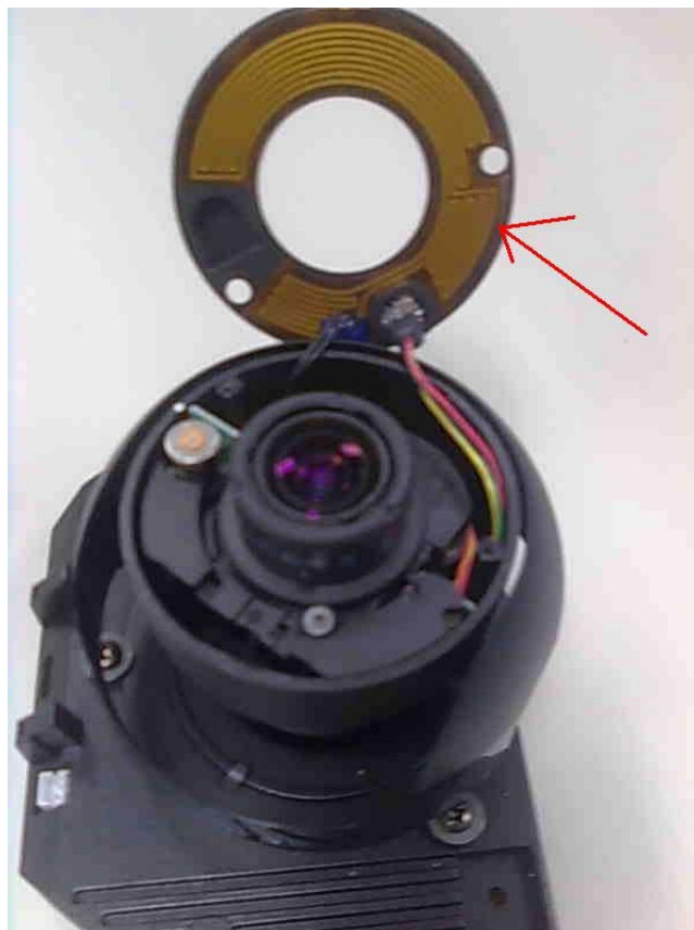
Photographs ID 3-16 heater view
