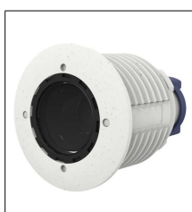
Mx-O-M7SA-8L040 120° 4K LPF Sensor Module WIDE M73/S74 sensor module with premium wide-angle lens, LPF special lens, e.g., for license plate detection (with infrared), aperture: f/1.8, max. image angle (HxV): 120°x60°, max. resolution: 4K UHD (3840x2160), IP66, white
